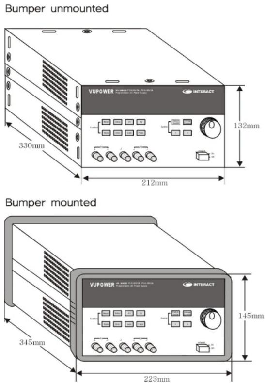
Figure 7-2. Dimensions of IPS-B Series DC Power Supply
