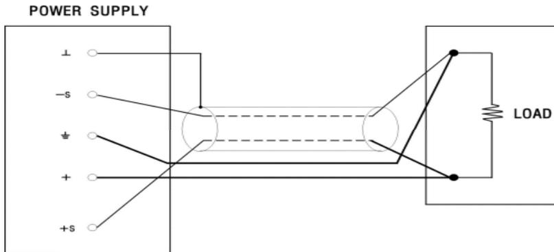
Figure 2-6. Remote voltage sensing connections
