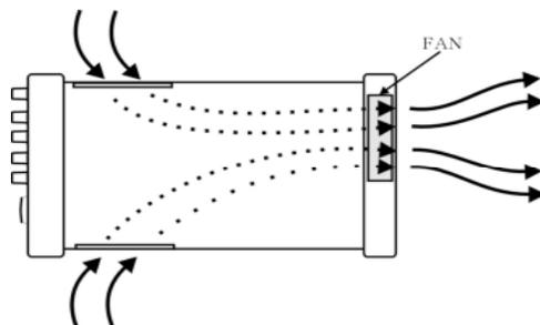
Figure 7-1. Cooling of IPS-B Series DC Power Supply
