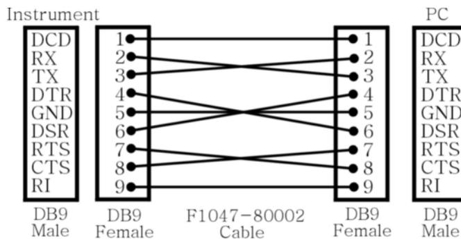
Figure 2-12. RS-232 Serial Connection
