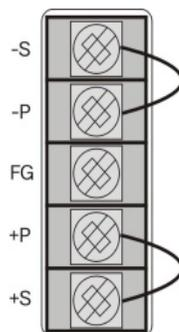
Figure 2- 7. Connection to the Rear Output
