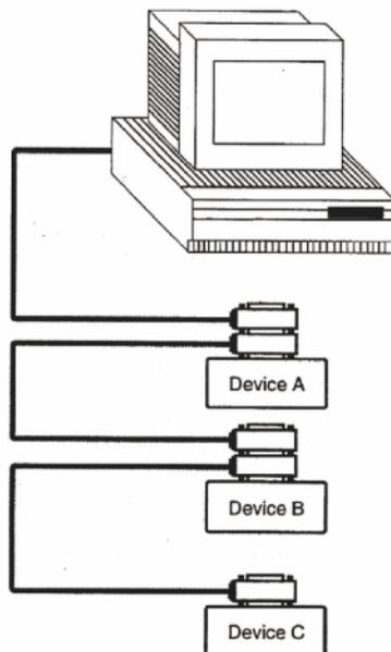
Figure 2-9. Linear Configuration
