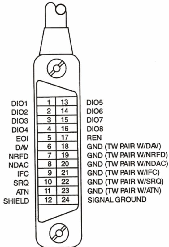
Figure 2-11. GPIB Connector and Pin Assignments
