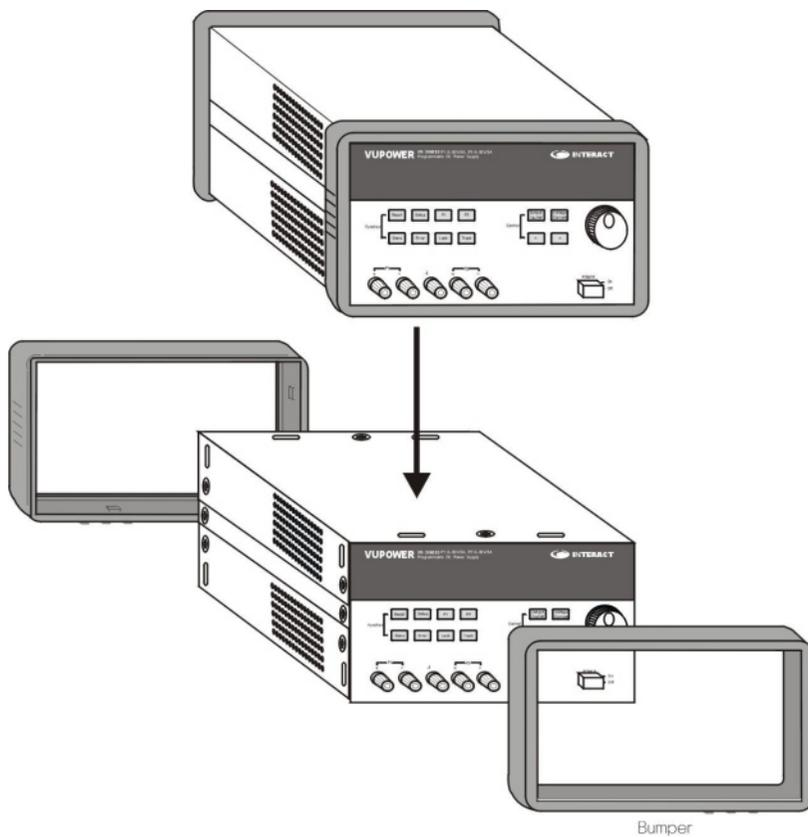
Figure 2-1. To mount the power supply on the rack.
